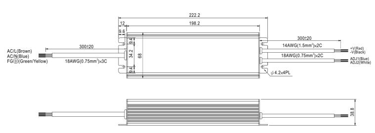
% IP67 rated. Output constant current level can be adjusted through output cable by connecting a resistor between ADJ1 and ADJ2.
